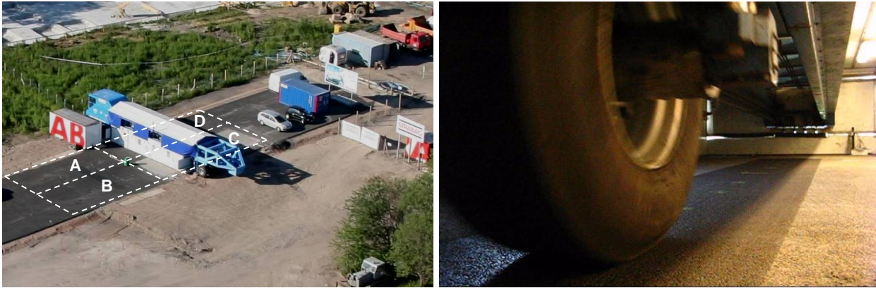
Figure 2: Heavy Vehicle Simulator HVS during testing of four types of asphalt pavements in 2008
