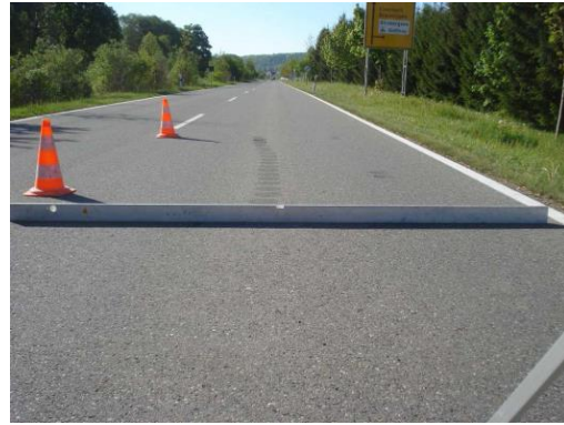
Figure 3: View of A/ section A and B/ section D, respectively without and with hydrated lime on the L181 test after 12 years. From [13].
