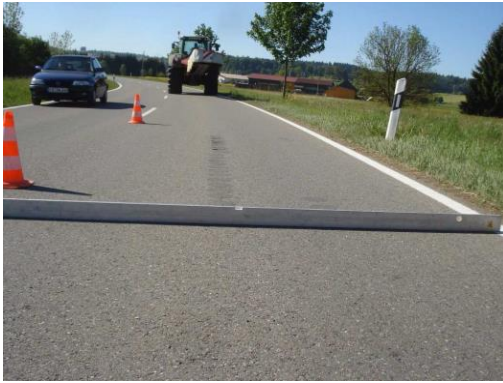
Figure 3: View of A/ section A and B/ section D, respectively without and with hydrated lime on the L181 test after 12 years. From [13].
