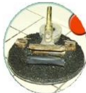
Photos 1 & 2: Benedict and Wet Track Abrasion Tests
