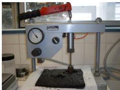
Photos 1 & 2: Benedict and Wet Track Abrasion Tests
