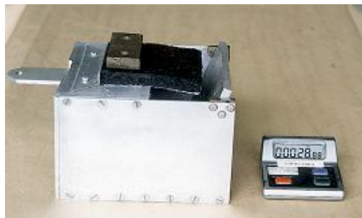
Photo 4: Hilt Cohesion Test
