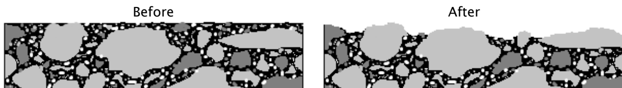
Figure 1: Pavement surface before and after exposure to studded tires
