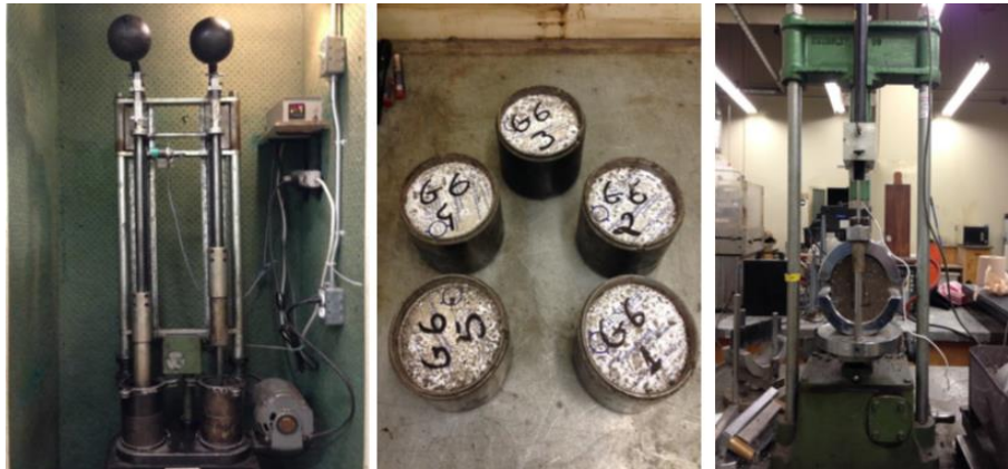
Figure 3: Marshall Stability test setup with Marshall Hammer, Compacted bricks, Marshall Testing (Left to Right)
