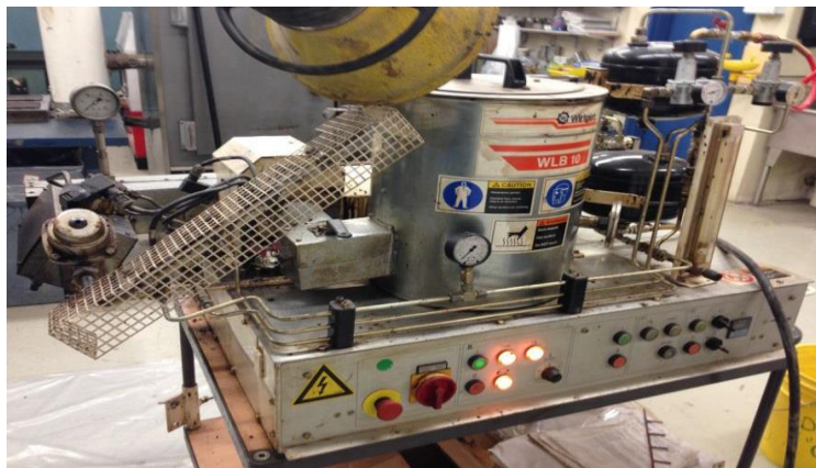
Figure 2: Writgen laboratory foaming machine at École de Technological Supérieure.
