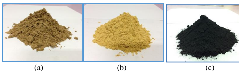
Figure 2.2: Walnut shell grinded and sifted through No 200 sieve (a), the images of apricot seed shell granule before (b) and after (c) the pyrolysis
