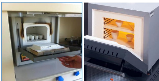
Figure 2.1: Placement of the crucibles containing the samples in muffle furnace and the process of pyrolysis [15]
