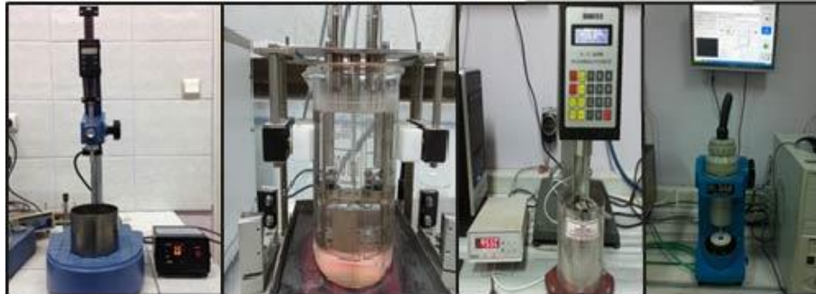
Figure 2.2: Penetration, softening point, viscosity and DSR experiment equipment.
