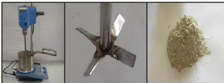
Figure 2.1: Modified bitumen mixture equipment and the montmorillonite used.
