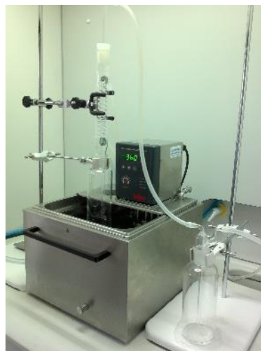
Figure 2: Laboratory reactor for continues bio-agent oxidation process
