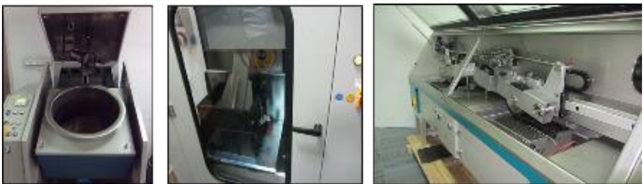
Figure 3: Pictures showing devices used in Hamburg rutting test.
