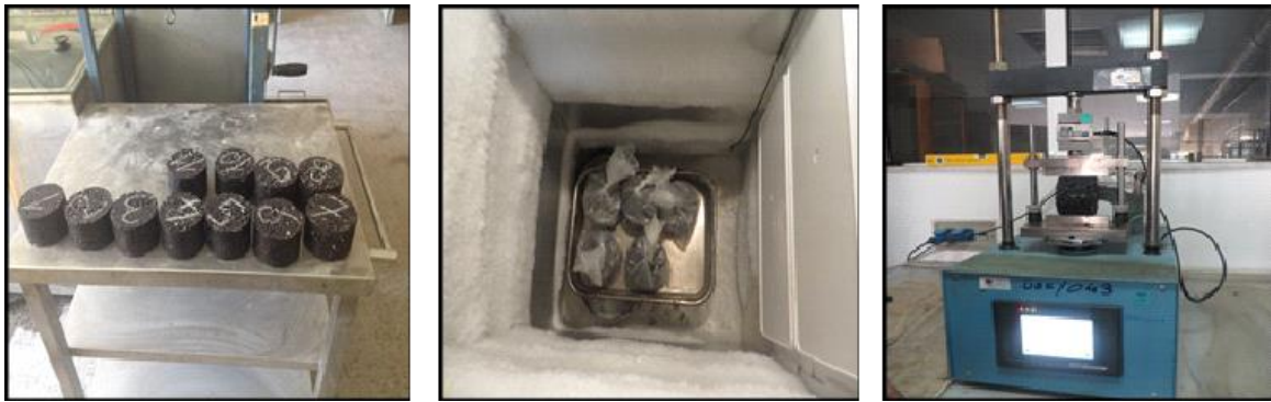
Figure 6: Pictures showing Indirect Tensile Test.
