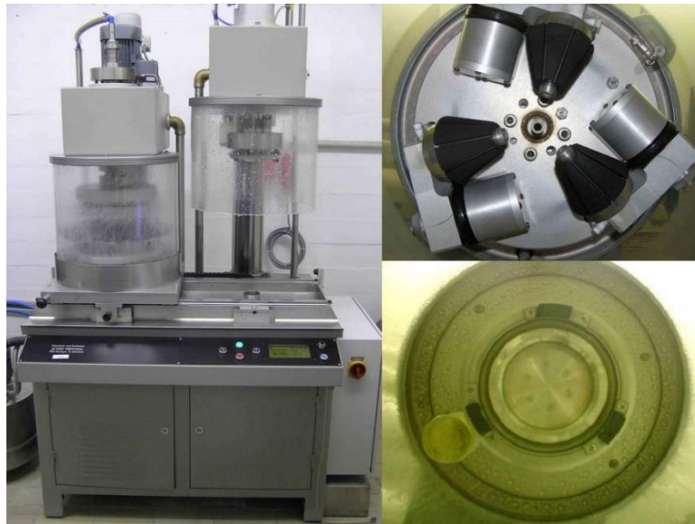
Figure 1: Wehner/Schulze test device at the Vienna University of Technology (left), polishing head (upper right), measuring head (lower right)
