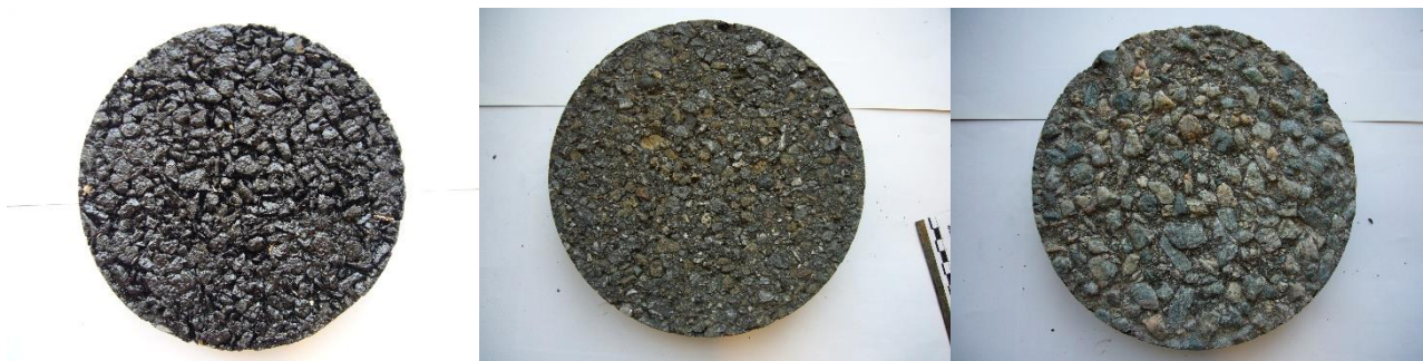
Figure 2: Test specimens - cores from laboratory-made slab (left) and asphalt pavements (centre and right)
