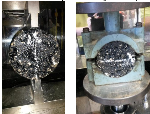
Figure 15: Self-Healing Asphalt Test.
