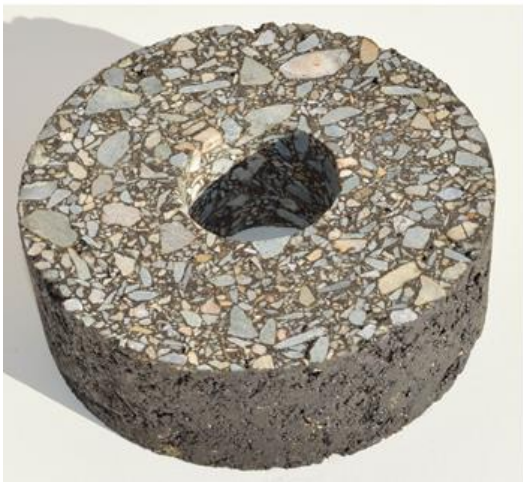
Figure 2: Uniaxial Shear Tester / top view, hollow cylindrical specimen, UST placed in UTM chamber/
