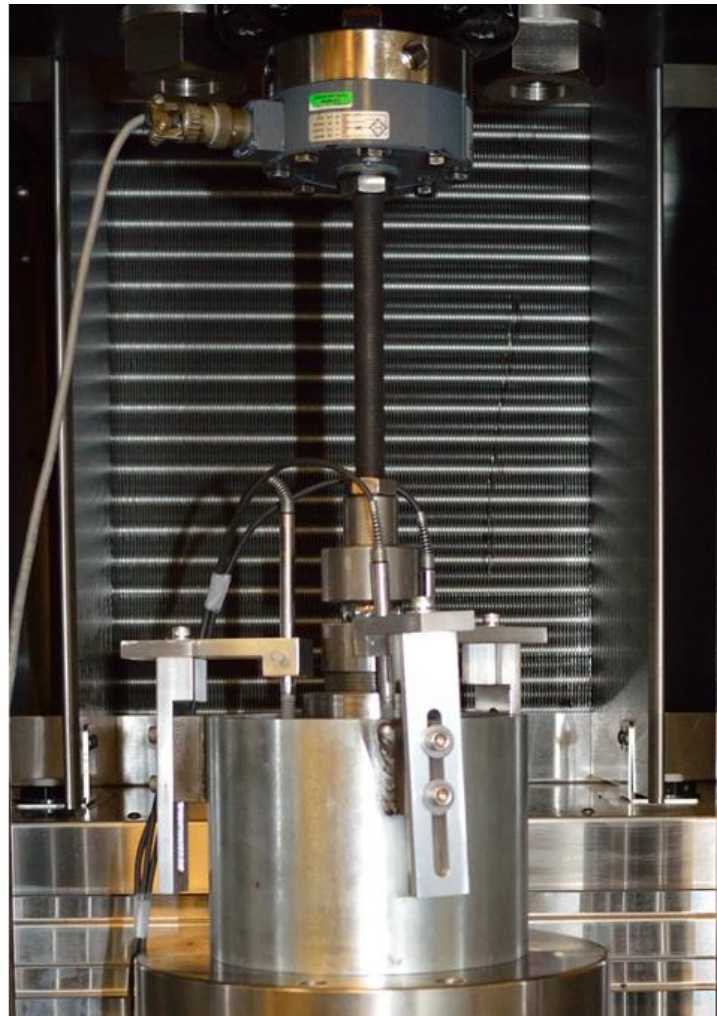
Figure 2: Uniaxial Shear Tester / top view, hollow cylindrical specimen, UST placed in UTM chamber/
