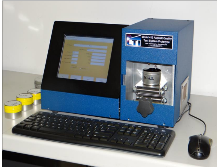
Figure 2: The first article prototype design of the bitumen QCT Device.
