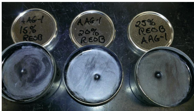
Figure 4: Indentations produced during typical testing with the QCT
