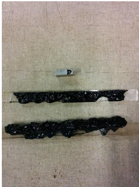
Figure 6: Failed attempt to mold BBR (AASHTO T 313) specimen from high content CRMB
