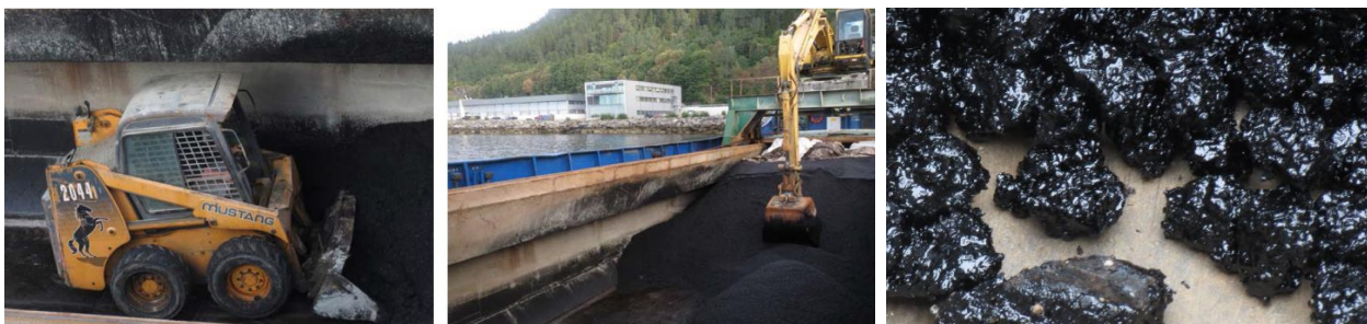
Figure 16: Cold asphalt gathered from the bottom and edges of the cargo must not be loaded onto the truck (Photo: Bjørn Hoven)
