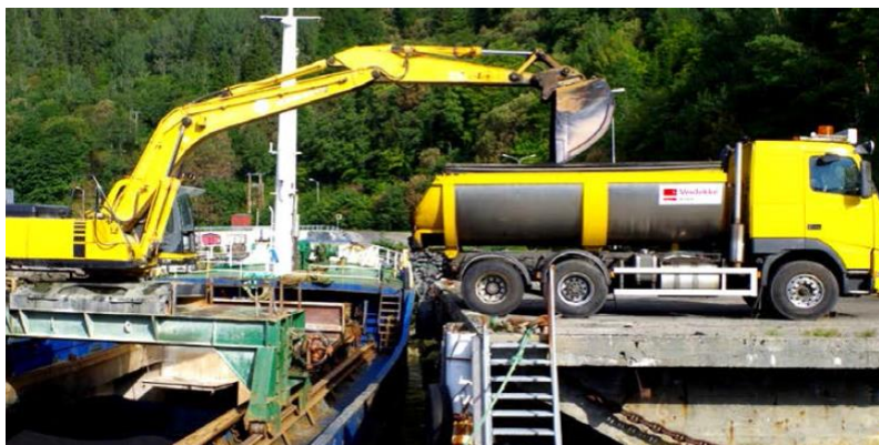
Figure 15: The truck should be perpendicular to the side of the boat during unloading (Photo: Marit Fladvad)
