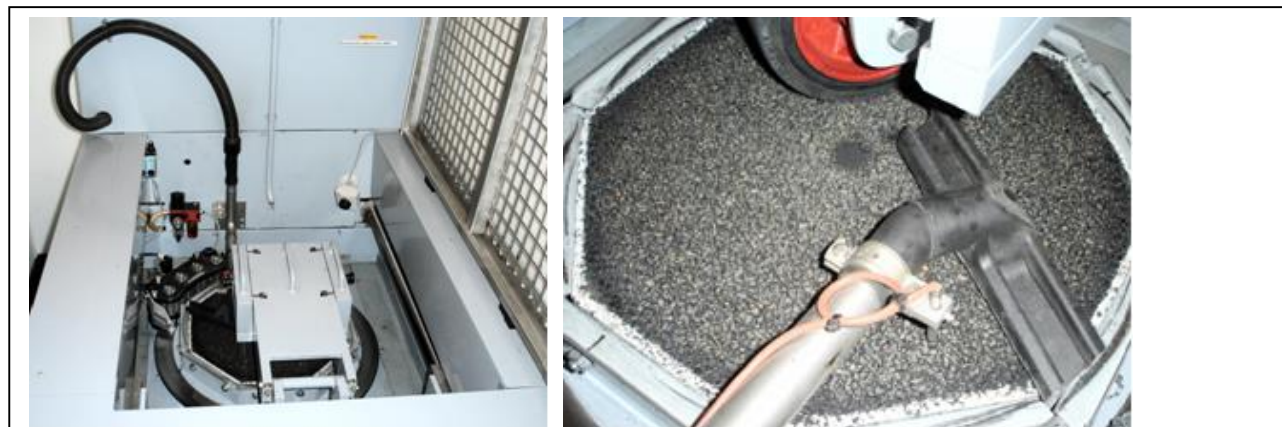
Figure 6: The Rotating Surface Abrasion Test device of Heijmans
