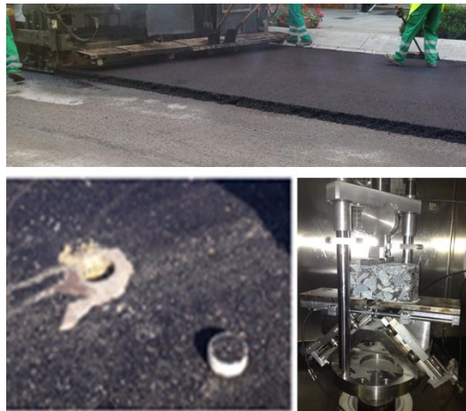
Figure 13: Detail of the evaluation of a cores obtained from an asphalt pavement using the UGR-FACT method.
