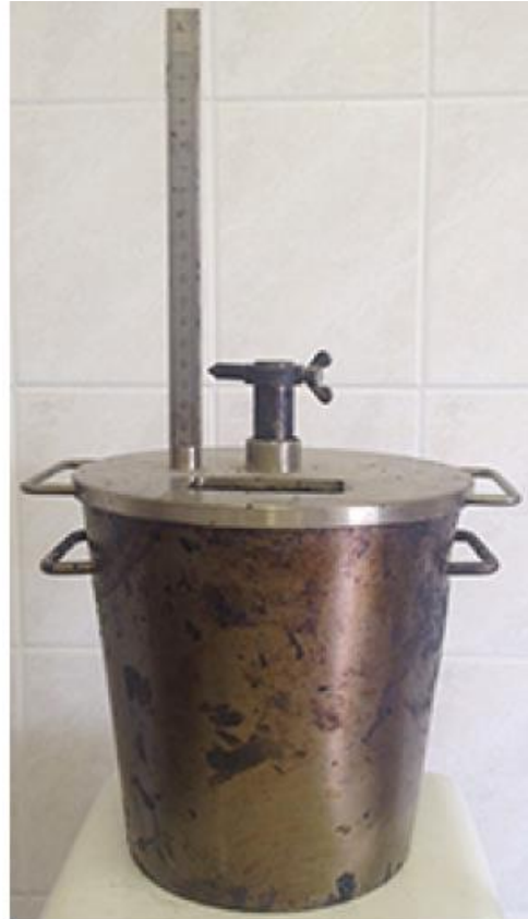
Figure 4: Test apparatus for workability determination [7, own photo]
