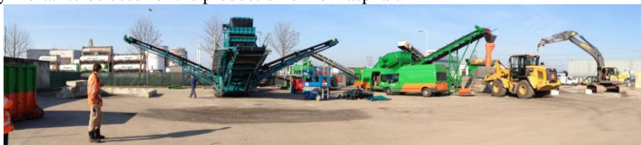
Figure 3: Full-scale decomposition of reclaimed asphalt
