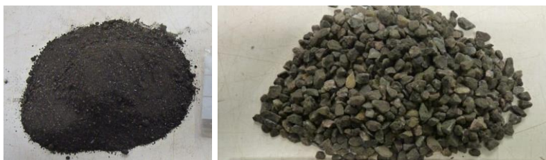
Figure 4: By decomposition of reclaimed AC new commodities become available. Left: mortar sand (sand, filler and bitumen), right: mineral aggregates in various fractions that hardly contain bitumen
