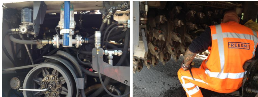
Figure 2: Left: water pressure and flow gauge mounted on milling machine. Right: inspection of chisel wear during measurements
