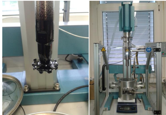
Figure 1: Cowles Agitator (Left) and Mixer Used (Right) for Blending Bitumen and Silane
