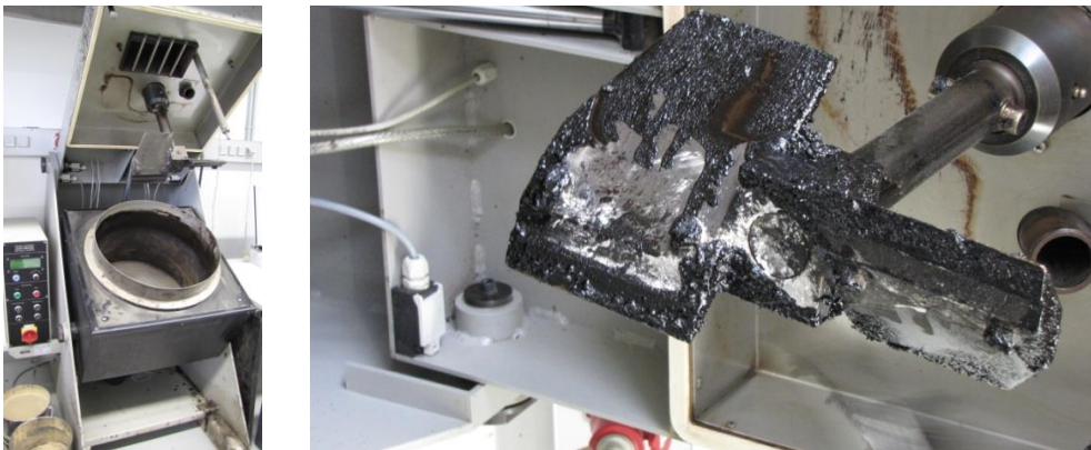
Figure 1: Opposite rotation pug mill used in this study.
