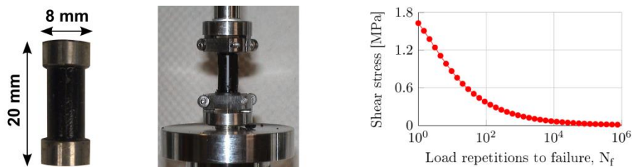
Figure 5: Bitumen column test specimen (left) [5]; Bitumen column DSR test setup (centre) [5]; Cohesion shear stress response transfer function at 25°C (right) [1].
