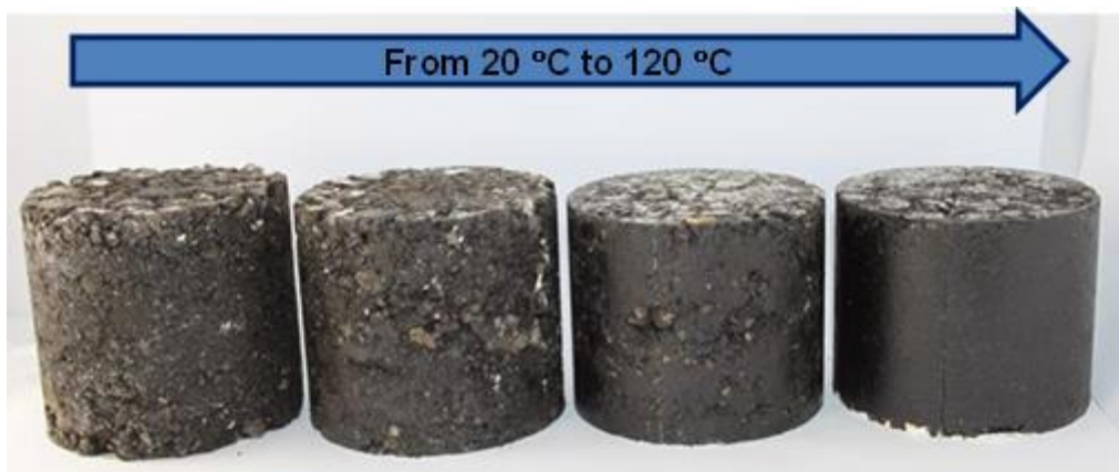
Figure 6. Aspect of the gyratory samples at 20, 40, 60 and 120 °C
