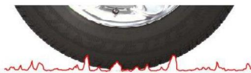
Figure 2: Positive texture of the road surface
