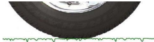
Figure 3: Negative texture of the road surface
