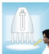
Figure 2a (left) en 2b (right): 2a. Luminance is a complex photometric quantity that represents what the human eye can observe. 2b. measuring luminance under a very small observation angle as the motorist sees a road.
