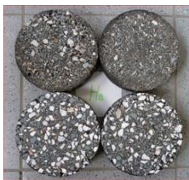
Figure 5: Comparison of the sawed lab. sample surface (beneath) to the original “outside” surface (above). The lab. sample surfaces show that in the outside surfaces there is more segregation of particles compared to the sawed surfaces.
