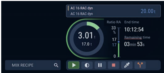
Figure 4: Digital management of an asphalt mixing plant with as1 control system.
