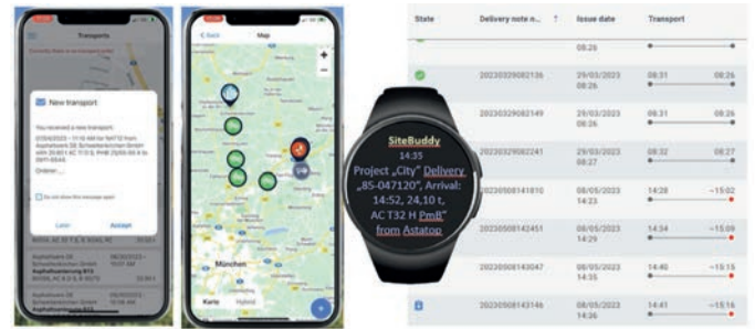
Figure 6: Digital transport information, positions of the trucks, mobile information about delivery with Q Transport and Q Site.
