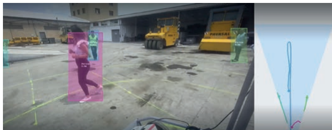
Figure 9: Person detection standing/running and trajectory relative to the machinery.
