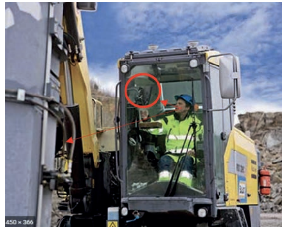
Figure 3: Image system in mobile machinery, diverting the operator's attention.
