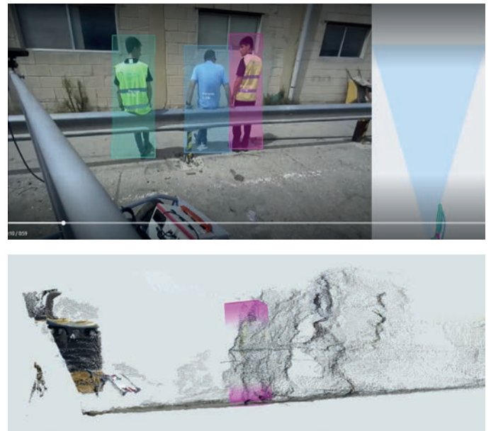
Figure 8: People detection and point cloud.
