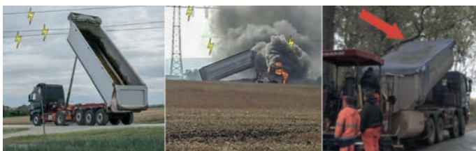
Fig. 6: Increased work safety with a push-off trailer compared to a dump truck
