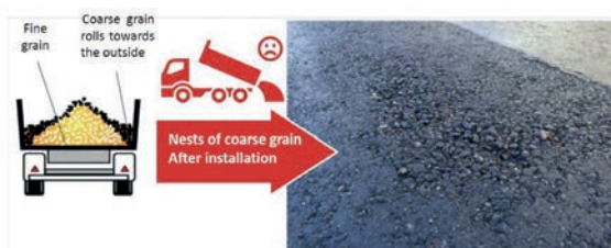
Fig. 1: Coarse grains roll outward – coarse grains come out first → clusters of coarse grain usually occur at intervals. Source: TU Darmstadt / FH Köln / Research project PAST (Prozesssicherer Automatisierter Straßenbau).
