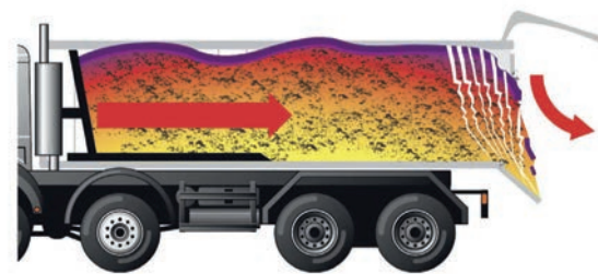
Fig. 7: Continuous mixing throughout the unloading process.
