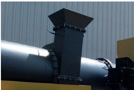
Photograph 5: granulometric classification of the RAP and incorporation into the mix.
