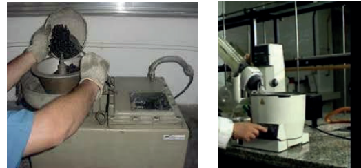
Photograph 7: Determination of binder content of the RAP.
