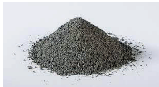
Predigested NFVU powder passes ASTM 20 mesh (0.841 mm)
