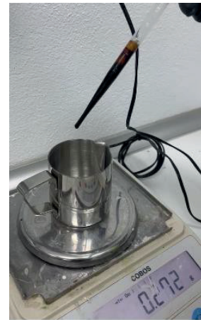
Photograph 12: Incorporation of the dose of BIOROAD WARM MIX, in the bitumen in the laboratory
