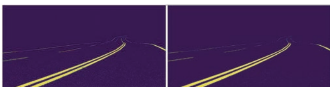
Figure 8. Image after mask application (left) and filtering and cleaning after erosions (right)
