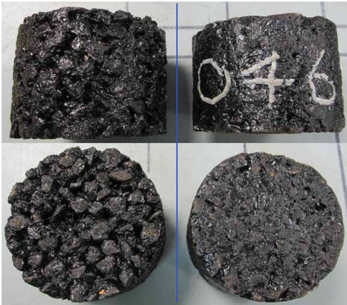
Figure 15 – Surface of SMA10 Pats: Gyropac @ 80 (Left) & 350 (Right) Cycles
