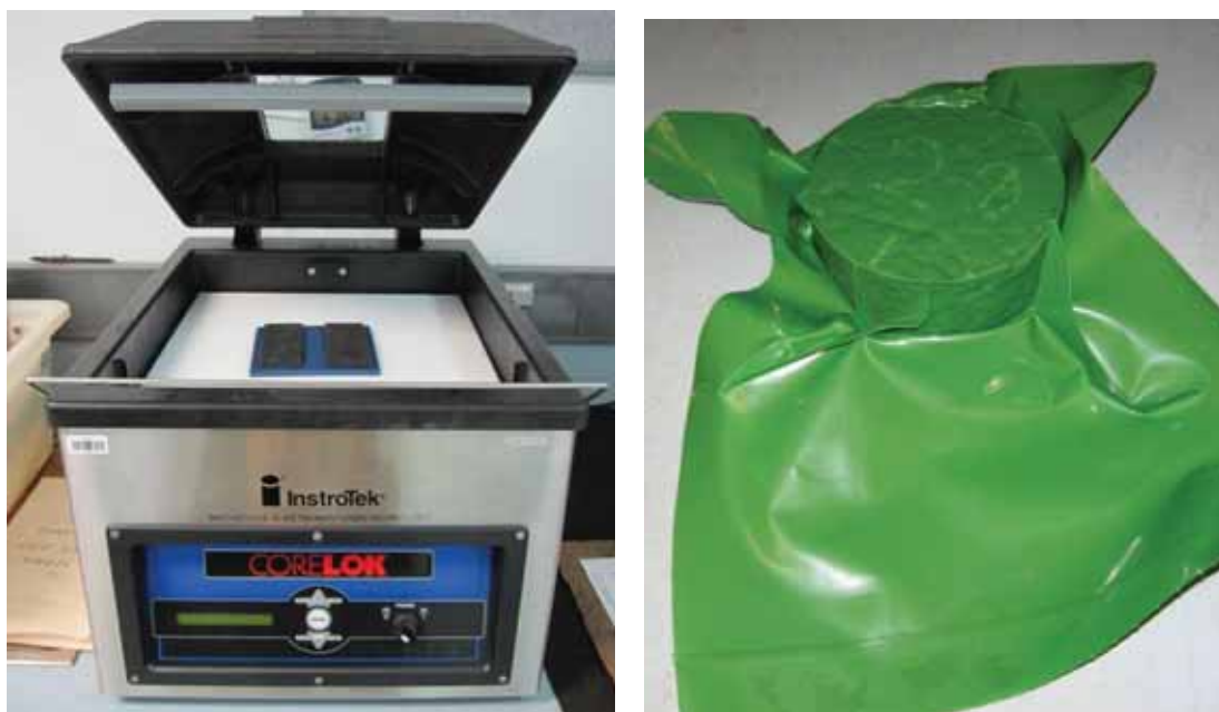
Figure 2. Vacuum Sealed Machine & Sealed Sample (Polymer Bag)
