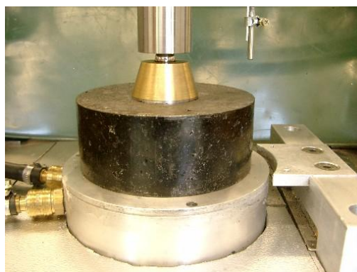
Figure 8: Setup for the uniaxial cyclic compression test with some confinement for mastic asphalts (UCCTC)
