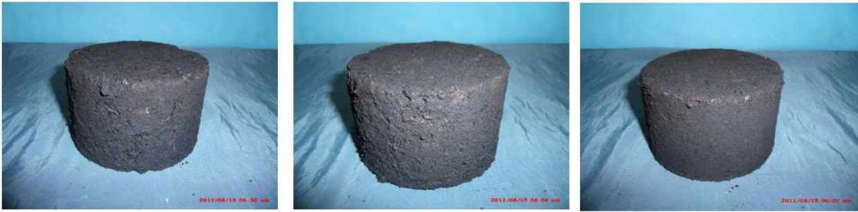
Figure 8: Typical performance of Marshall cores made with asphalt mix with plant mix additive after soaking in Kerosene for 24-hours
