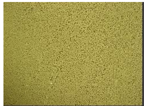
Picture 1 : Polymer network in a cross-linked elastomer modified bitumen
