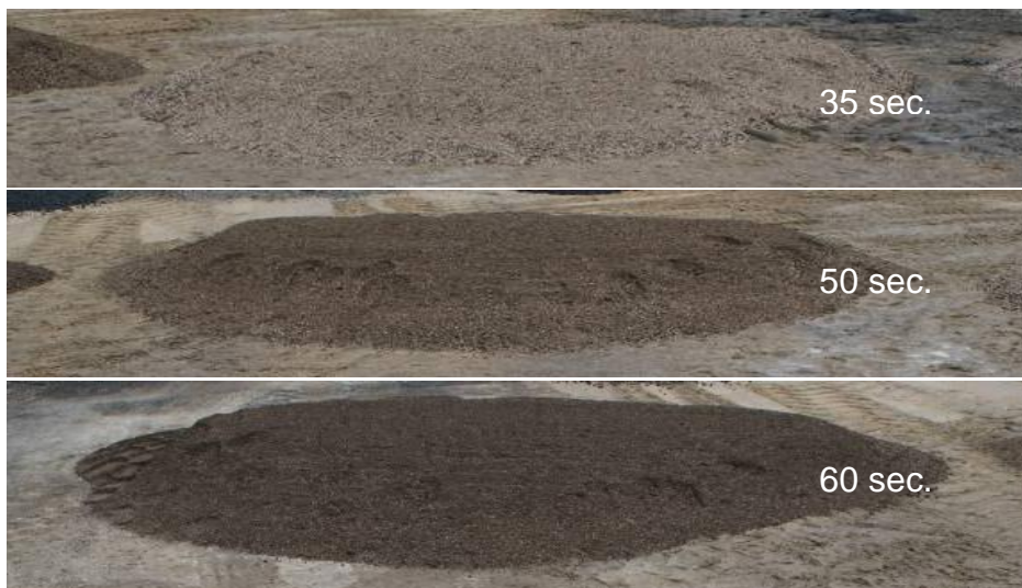
Figure 1: 25 % RAP, mixed with superheated light coloured virgin aggregate The visible difference in colour of the batches can be used to assess a mixing time to achieve good commingling of RAP binder with virgin binder
