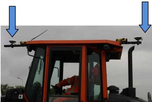
Figure 6: Two GPS rovers on a tandem roller (to measure crabwalk)
