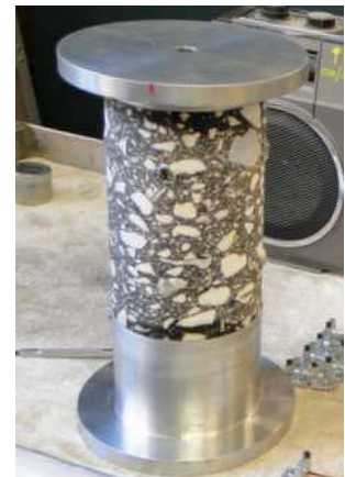
FHWA HRC AMPT test*
