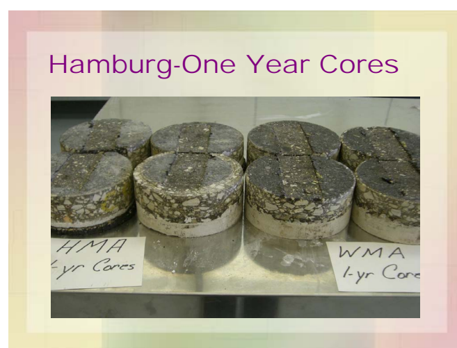
Testing of WMA and HMA by TxDOT
