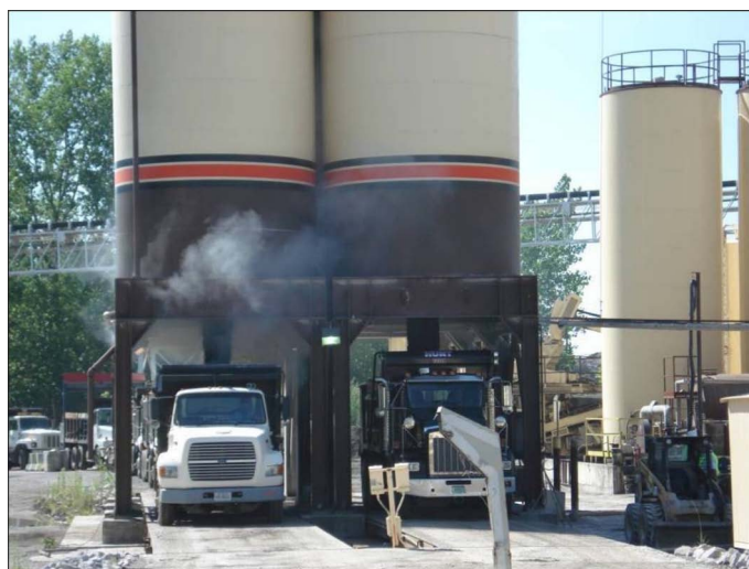
HMA on left and WMA on right being loaded from storage bins.
