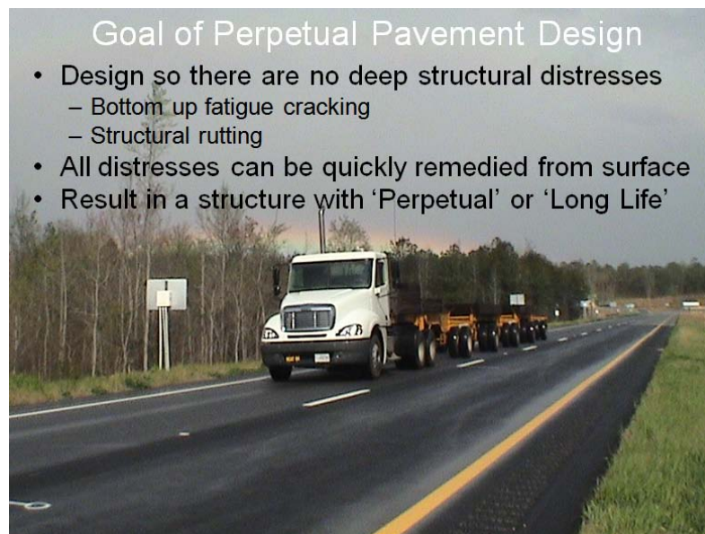
NCAT test track providing field proof for very long life flexible pavements
