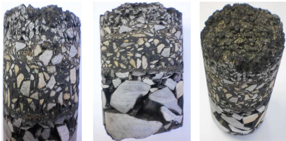
Figure 10 : Example of Asphalt Cores
