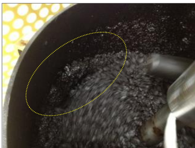
Figure 9: Deposition of fine material on wall of mixing bowl
