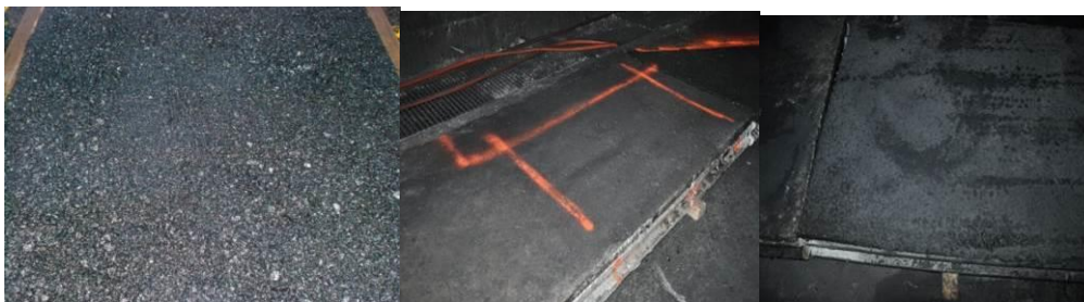
Figure 15: Surface appearance of the bituminous mixture: Before the test (left); white sample after the test (middle); sample that containing fire retardant after the test (right).
