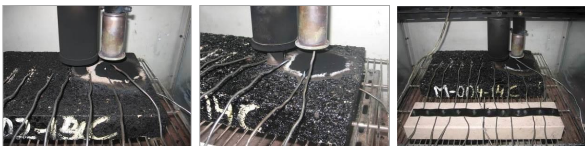
Figure 6: Appearance of the specimens after the test. No additive (left) 1.0 % (center) and 1.4 %(right).
