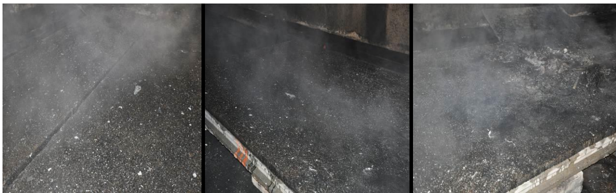
Figure 21: Bituminous mixture surface after test with a burning car.
