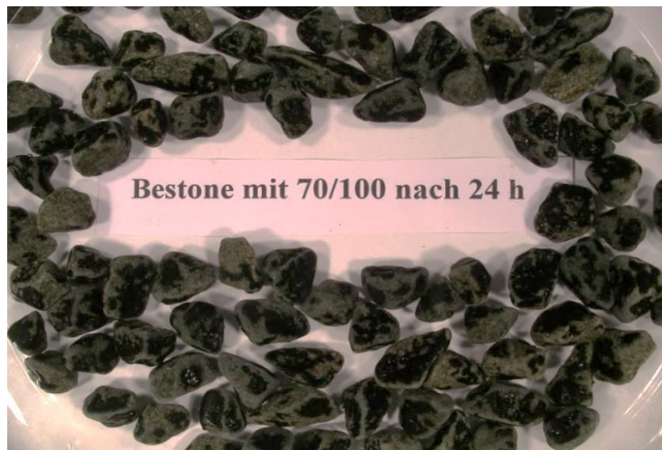
Figure 3 Bestone with 70/100-bitumen after 24 hours Rolling Bottle Test
