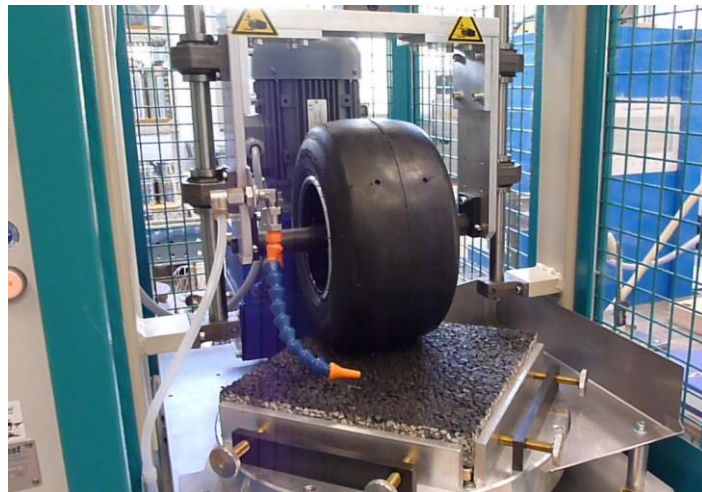
Figure 3: Experimental set-up of the ‘Darmstadt Scuffing Device’ (DSD) equipment at BRRC
