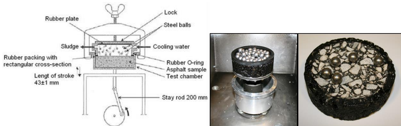
Figure 4: Prall apparatus (figure adopted from EN 12697-16:2004, photos by Brynhild Snilsberg)
