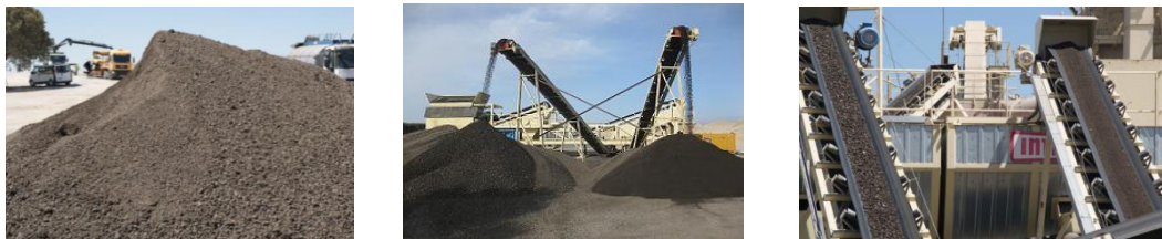
Figure 1: RAP classification into two fractions.
