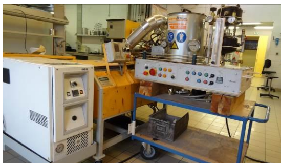
Figure 5: Pilote WLB 10 and pug mill for manufacturing foamed asphalt mixes in the laboratory
