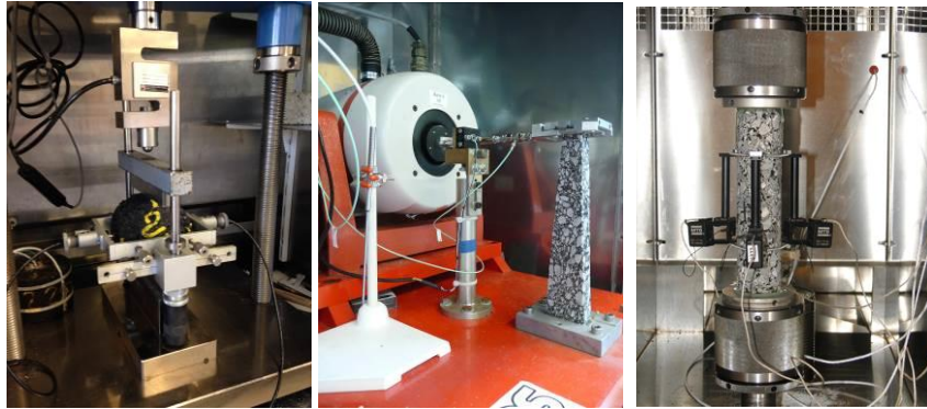
Figure 4: Modulus measurements, (b) Modulus and fatigue on trapezoidal samples, (c) TSRST
