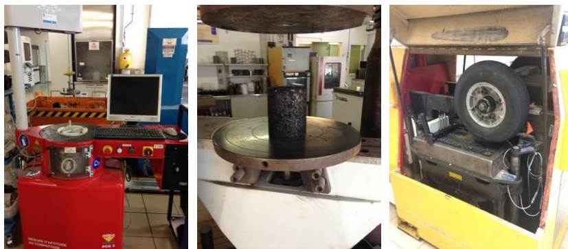
Figure 3: test conducted for general requirements: (a) gyratory shear compaction, (b) water resistance with Duriez, (c) rutting resistance on large device
