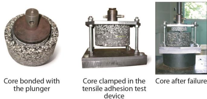
Figure 2: Tensile adhesion test device (TAT) and experimental setup
