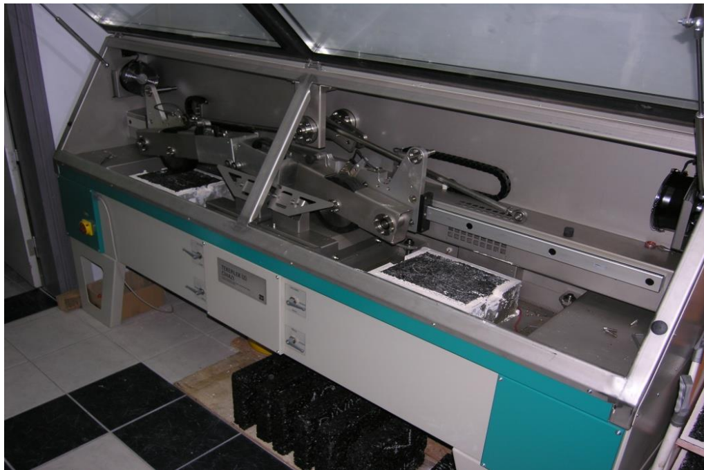
Figure 5. Rutting Test of Two Identically Plastered Specimens in HWTD
