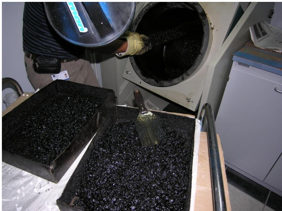
Figure 3. Mixing stage of aggregate and bitumen
