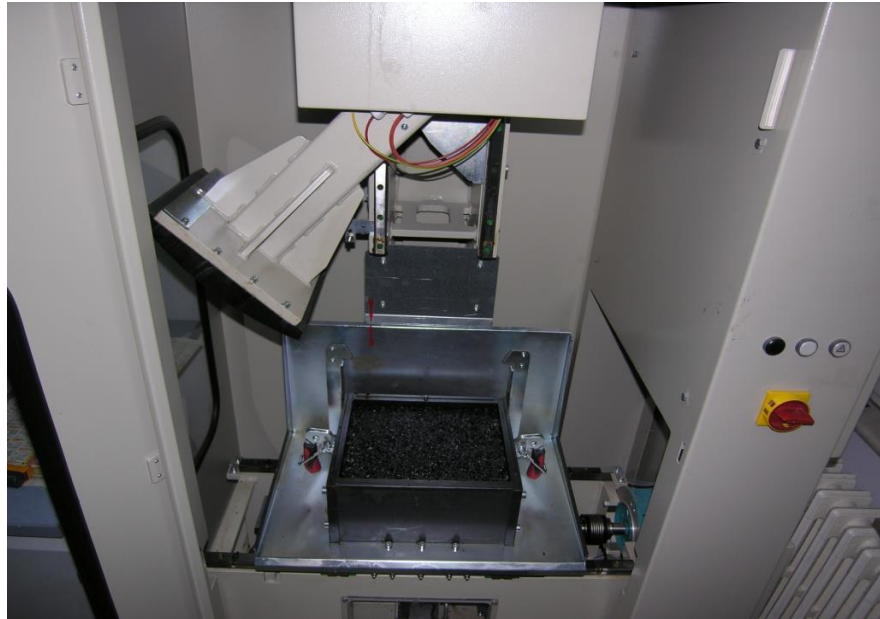
Figure 4. Compaction of slabs in segmental compactor
