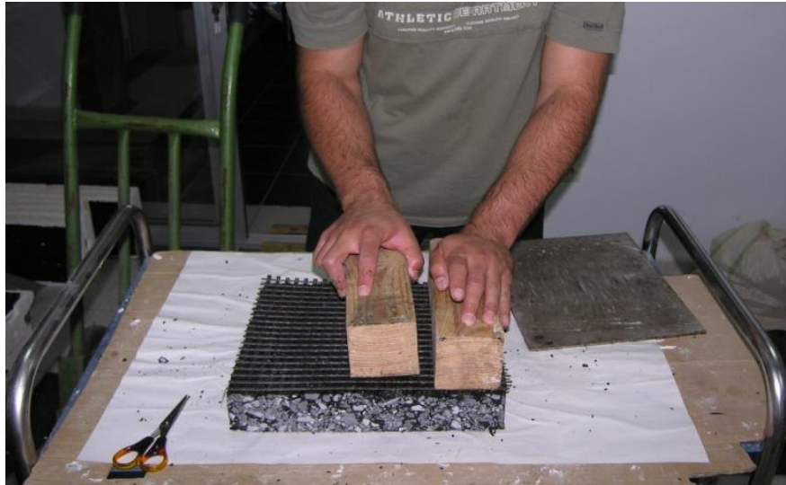
Figure 2. Preparation of specimen for test: Installing of geosynthetics
