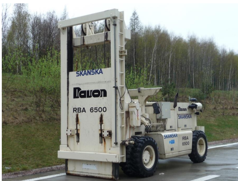
Figure 6: Drop hammer – machine for PCC pavement segmentation
