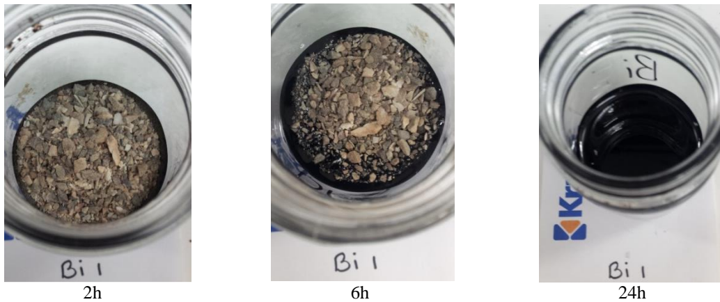
Figure 7: Surface of bitumen with crushed stones after 2-24h at 40 °C
