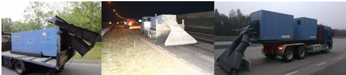
Figure 1: Special equipment used for Modimuls ZV : the air-jet turbine motor [2]
