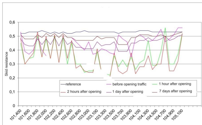
Figure 4: Results of skid resistance measurements during 7 days after the treatment for A15 [3]
