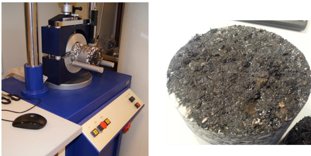
Figure 7: Shear bond test (EN 12697-48). Tested specimen; poor bonding caused by wet and dirty surface.
